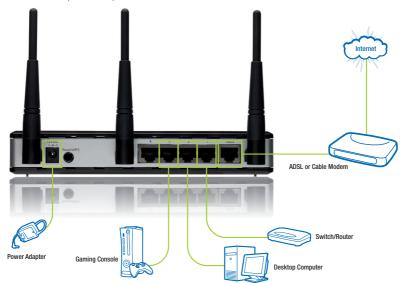
Please check all LEDs on the front panel. 'PWR' LED should be steadily on, WAN and LAN LEDs should be on if the computer / network device connected to the respective port of the router is powered on and correctly connected.
